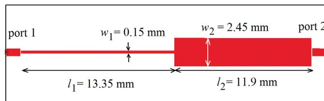
Fig. 6. Microstrip implementation of a stepped impedance resonator in TMM10 (thickness 0.635 mm) with  $\eta = 4$  and  $\nu = 1$  for resonant frequency 2.3 GHz.
