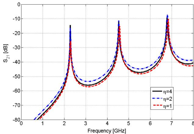
Fig. 8. Variation of the transmission factor  $S_{21}$  due to different  $\eta$ , calculated by Sonnet for case  $\nu = 1$ .
