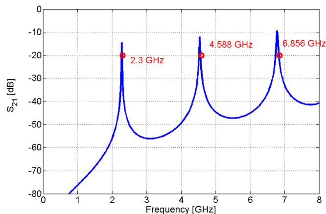
Fig. 7. The transmission factor  $S_{21}$  calculated by Sonnet (solid line) and the resonant frequencies predicted by analytical approach (o in red), for case  $\eta = 4$  and  $\nu = 1$ .
