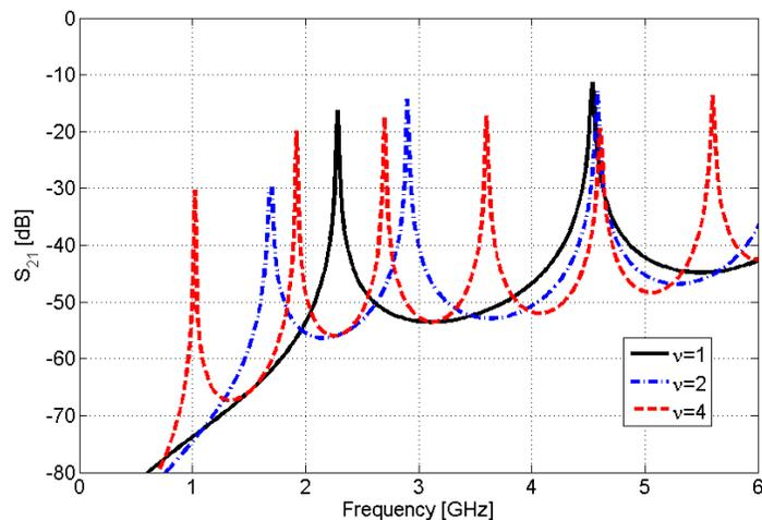
Fig. 9. Variation of the transmission factor  $S_{21}$  due to different  $\nu$ , calculated by Sonnet for case  $\eta = 2$ .
