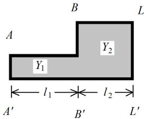
Fig. 1. Stepped Impedance Resonator (SIR) consists of two microstrip lines with characteristic admittances of  $Y_1$  and  $Y_2$  and lengths  $l_1$  and  $l_2$ .
